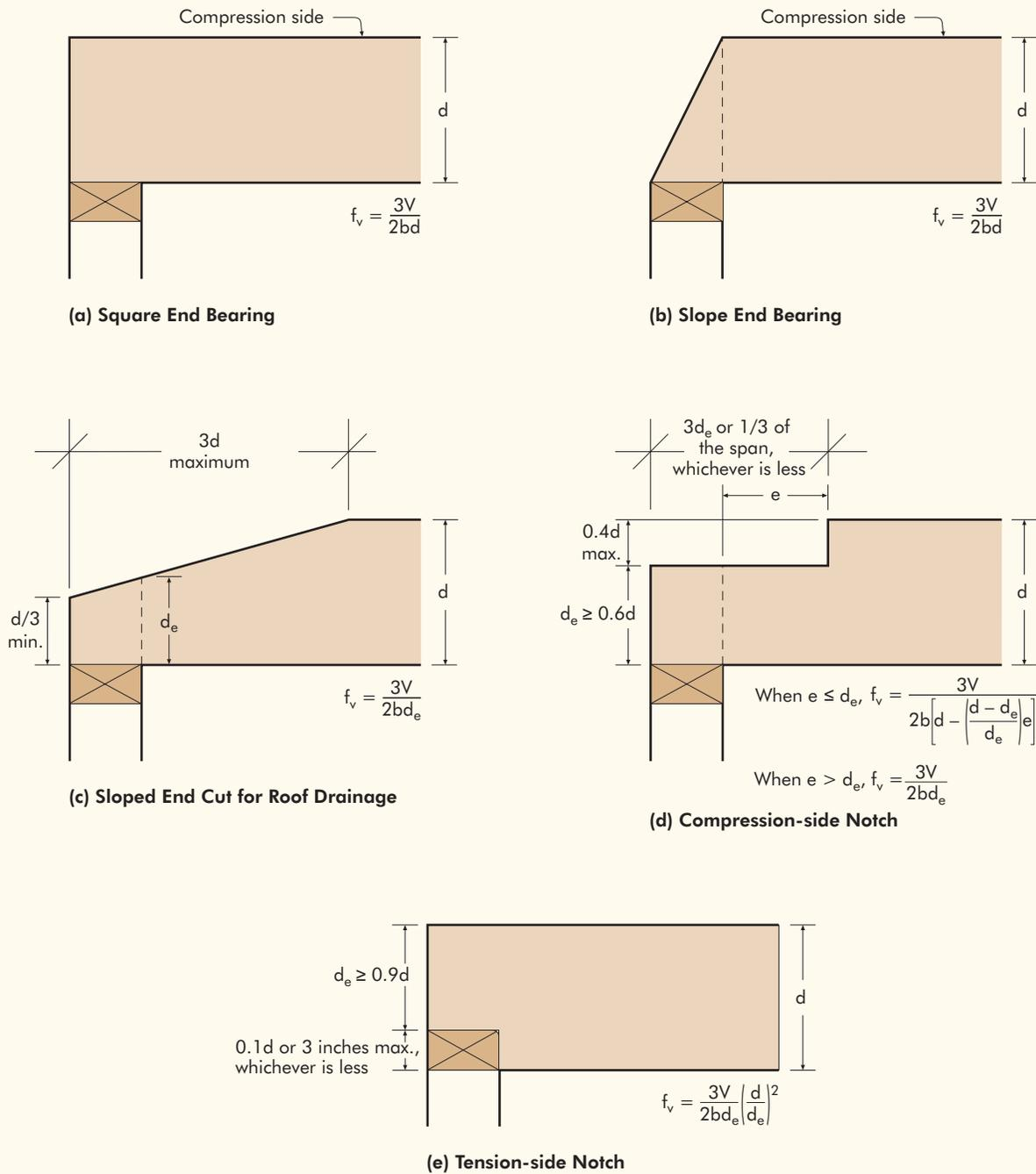
$f_v$  = shear stress (psi)       $V$  = shear force at notch location (lb)       $b$  = width of beam (in.)
