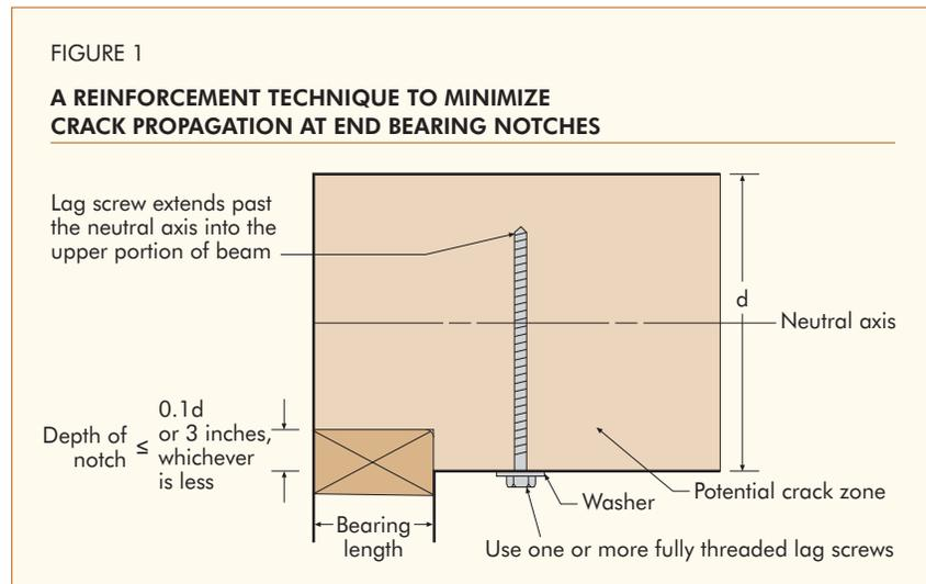
This procedure can also be used as a field remedy to minimize further propagation of an existing crack.
